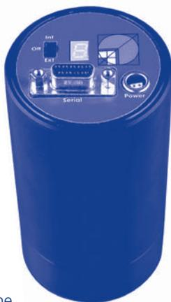
The temperature range: 1 mK to 100 mK. Use is commonly limited to a maximum ~ 50 mK because of the long integration periods necessary at higher temperatures). This is the primary technique used by Oxford Instruments at millikelvin temperatures. Nuclear orientation thermometry may be used to calibrate much faster thermometers, like Pt-NMR, PdFe susceptibility, carbon or  $\text{RuO}_2$  resistor thermometers.
