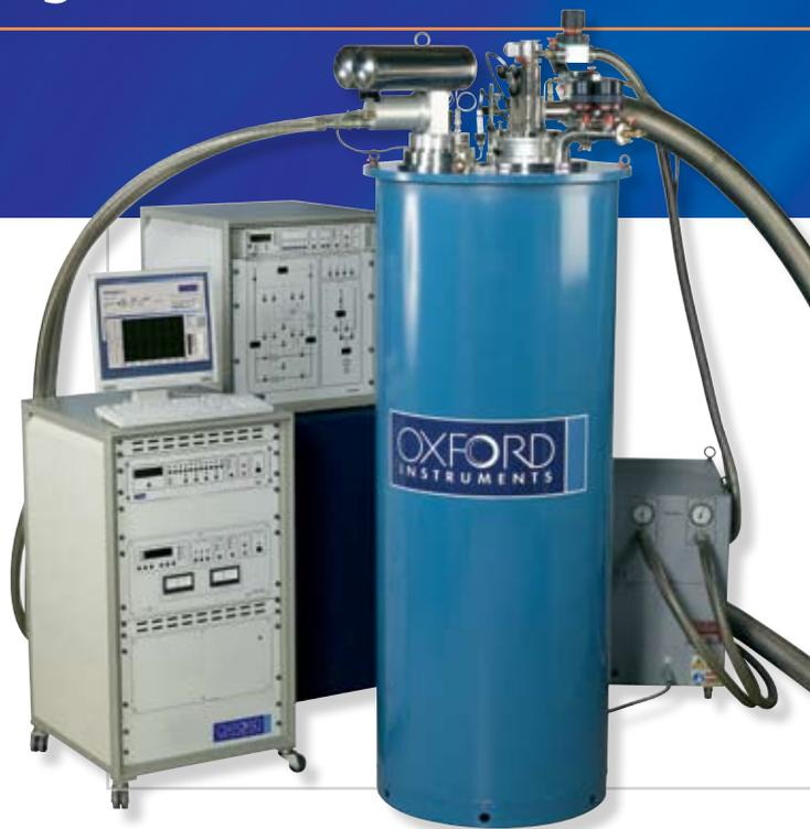
Recondensing dewars use a cryocooler to capture evaporated gas and turn it back into liquid helium. Using recondensing technology considerably decreases the helium consumption of these magnets. The cryostat is filled once with liquid helium, then the system can be kept cold continuously with virtually no helium consumption.
