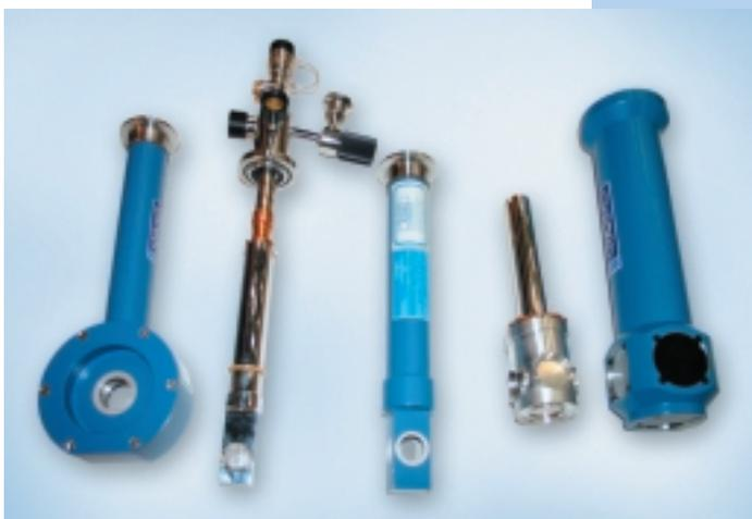
From left to right: Interchangeable MicrostatHe tail, cold unit fitted with the MicrostatHe radiation shield, MicrostatHe Rectangular tail, OptistatCF-V radiation shield and OptistatCF-V tail.
